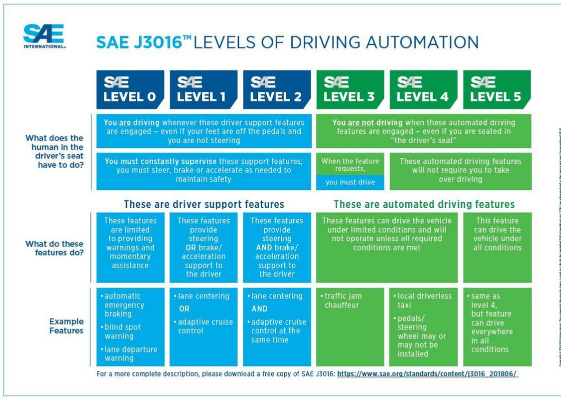
Figure 7. Levels of Driving Automation (Credit SAE)
