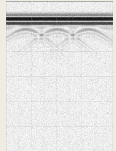
GPR image shows the b-scan which resulting from 3 pvc pipes without leakage
